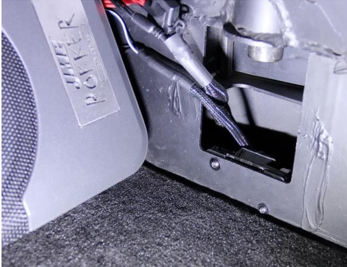
**Step19A-Carmel:** Slide the subwoofer into its left mounting position and hold in place as you mark/punch the location for the 4 mounting holes in the rear firewall. Then remove the subwoofer and drill these 4 holes using a 7/32" drill bit.
