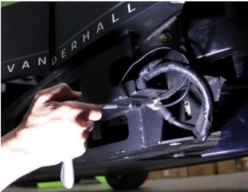
**Step15A-Carmel:** Route the subwoofer wiring harness, starting from inside the left rear storage compartment, down thru the circuit breaker access opening, down thru the grommet, and forward along the body thru to the upper engine cowl location. (Follow the routing of the ground strap)
