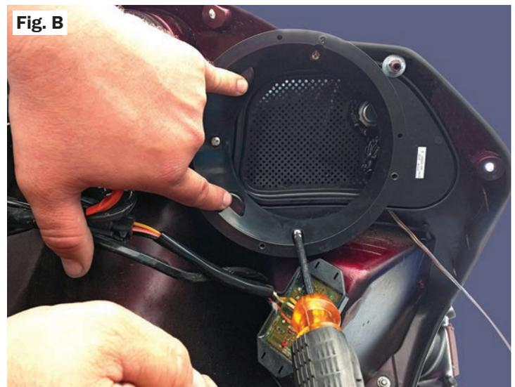
10. Then connect the terminals from the speaker wires of your audio system to the correct spade terminals on the wire leads from the ROKKER speaker grills.
