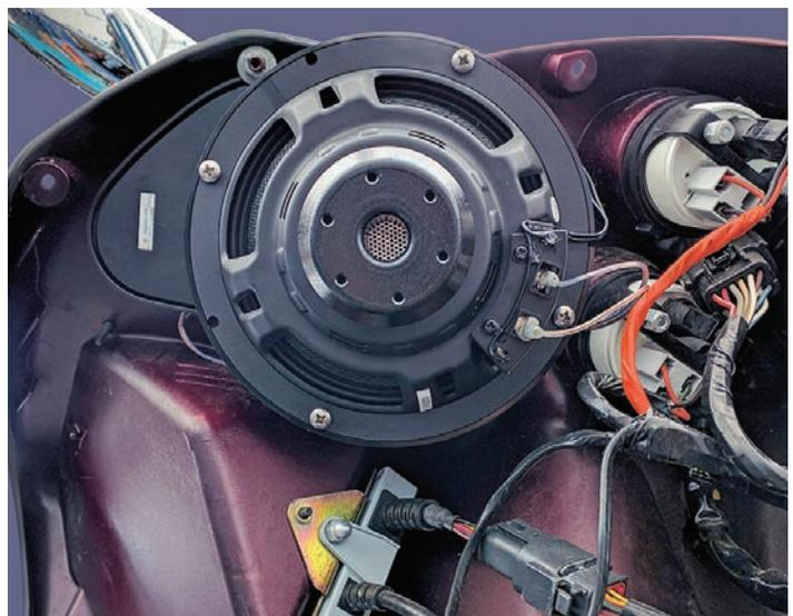
**Important Note:** 2012-2013 CVO RoadGlides come from Harley with smaller 5X7" stock speakers installed. Therefore to install the custom J&M ROKKER XXR series 6.71" speakers into the fairing, you will need to obtain from Harley, the replacement speaker/grill adapters, Harley part# 77021-98B (right side) & 77022-98B (left side), or J&M part# RRP-ARGSPA.
