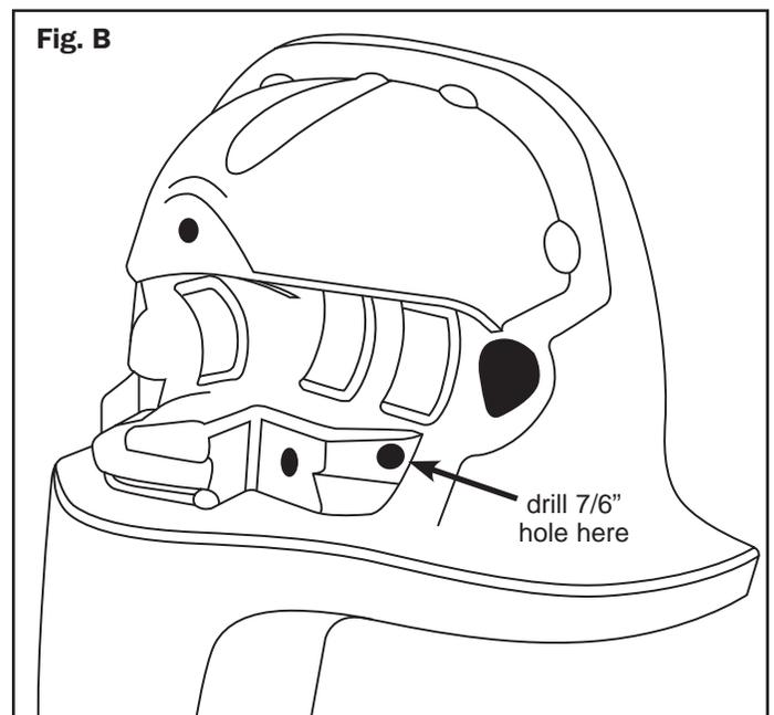
7. Install the new left and right-side housings using the provided panhead Philipps screws in place of the Torx screws that were removed.
