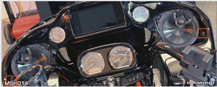
Step 9-Remove the last two T25 screws. Hold the fairing steady during the disassembly process to prevent it from falling off.
