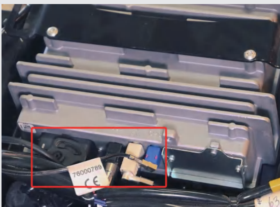
Step 11-Now, we need to remove the factory connector on the back of the radio. There is a small button on it. First, press the button, then slide it downward until it is unlocked, and finally pull it out. Remove the other cable interfaces to take out the radio.
