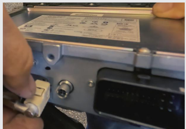
Step 11-Now, we need to remove the factory connector on the back of the radio. There is a small button on it. First, press the button, then slide it downward until it is unlocked, and finally pull it out. Remove the other cable interfaces to take out the radio.
